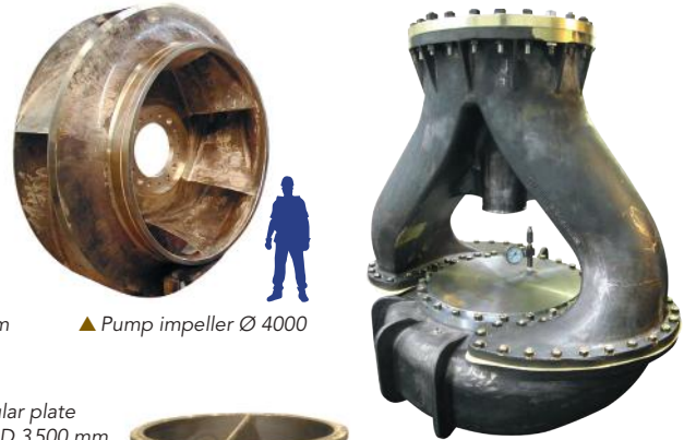
▲ Pump in hydro test 2000kg height 3600mm
