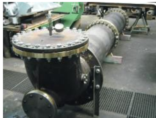
▲ Pump in hydro test 3500kg height 5800mm
